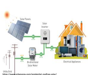
Grid-connected rooftop solar systems
